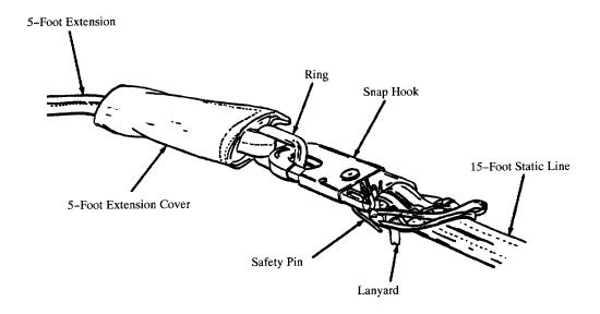
b. Slide the cover that is permanently attached to the standard 5-foot extension down over the snap hook of the standard 15-foot static line, and tie and tape in place using 2-inch wide masking tape.
