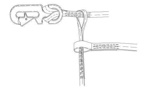
d. Continue passing the snap hook through the 3½-inch loop until a taut girth-hitch is made securing the 5-foot extension to the 15-foot static line. (There will be a half-twist in the 3½-inch loop when forming the girth-hitch.)
