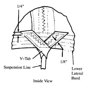
V-Tab Ends Secured To Lower Lateral Band
