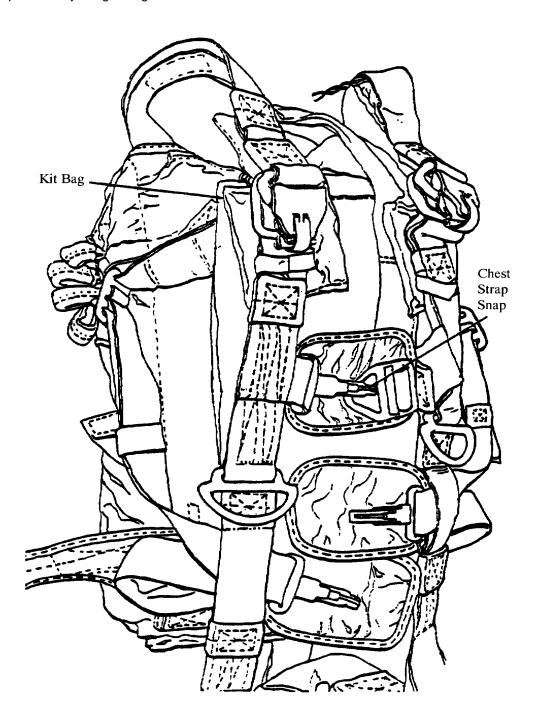
2. Pull the leg-strap through the kit bag carrying handle, under the diagonal back-straps; criss-cross the leg straps, and attach the quick-ejector snap to the adjusting V-ring.
