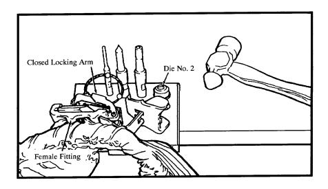
b. Center the No. 1 disassembly punch on the rolled end of the assembly pin. Strike several blows with an 8- to 12-ounce hammer to break off the riveted head of the pin. Drive out the assembly pin.
