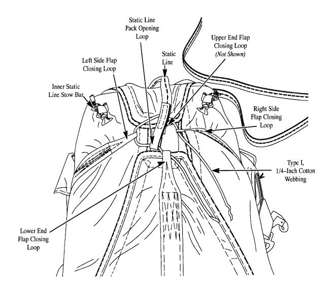
6. Pull loops close enough together to have an opening, of approximately 2-inches in diameter, between loops. Tie webbing with a surgeon's knot and a locking knot, making a tie between the right side flap and the lower end flap closing loops. Cut webbing approximately 2-inches from the knot. Keep the remaining lengths for the next connector link ties.
