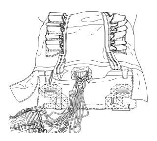
4. For the standard static line, double a 36-inch length of Type I, ¼-inch, cotton webbing. Pass one end of the doubled webbing through the static line buffer loop, through the bridle loop of the canopy, and back through the static line buffer loop.
