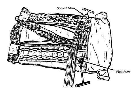
15. Continue alternating the stows from right to left until approximately 8- to 10-inches of suspension lines are left unstowed.
