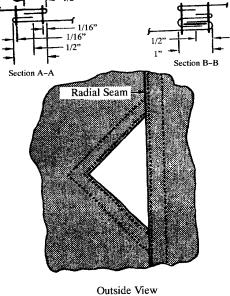
(D) Triangular Patch Including Radial Seam, Noncontinuous-line canopy.
