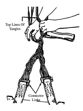
(3) Pull the risers, or pack assembly, through the opening. Do not permit risers, or pack assembly, to turn.
