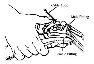
d. Operate latch and check for smooth operation. Close and lock latch.
