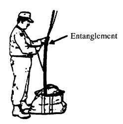
6. After the suspension lines have been cleared, the No. 2 person may hold, or temporarily secure, the pulley rope while the No. 1 person proceeds to clear debris from other parachute components such as the risers, harness, and pack tray.
