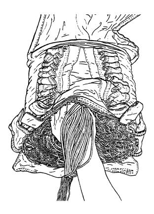
7. Turn the deployment bag upright, with the static line end down. When the entire canopy and net are stowed, the suspension lines should be centered on top of the deployment bag.
