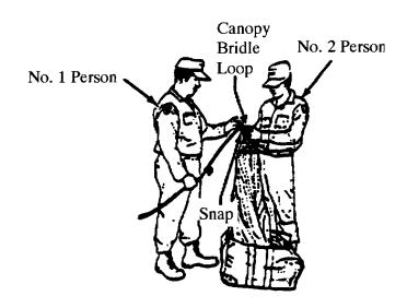
2. Through use of the pulley rope, the No. 2 person will raise the canopy to a suitable height; this will enable the No. 1 person to perform shakeout on each of the canopy gores. Until the gore shaking process is completed, the No. 2 person will maintain a steady pull on the pulley rope to hold the suspended canopy at the working height needed by the No. 1 person.
