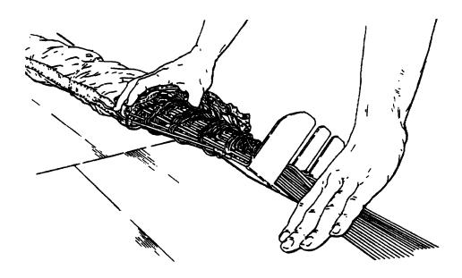
12. Place packing weight on suspension lines next to the separator.
