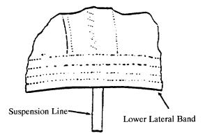
5. Center the new tab lengthwise under the suspension line, even with the lower edged of the lower lateral band. Wrap the tab tightly around the line, forming a V on the inside of the lower lateral band. Hand-tack the tab to the inside of the lower lateral band.
