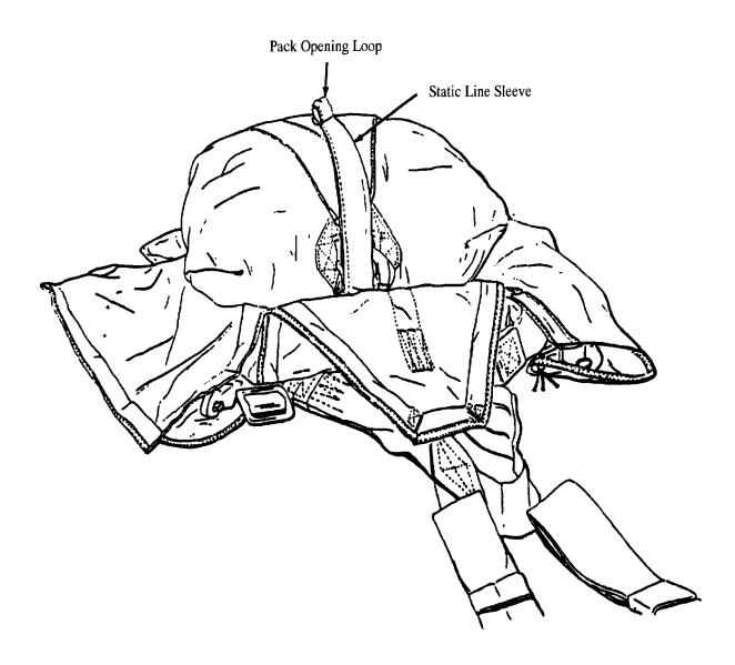
5. Lay pack-closing flaps over the deployment bag. Thread a 40-inch length of Type I, ¼-inch, cotton webbing through the lower end flap closing loop, the static line pack loop opening loop, the left side flap closing loop, the upper end flap closing loop, under the static line, and through the right side flap closing loop.
