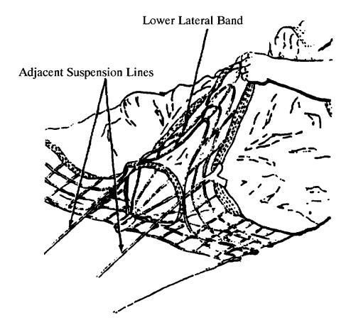
3. Reattach the canopy to the apex hook after the inversion is removed.
