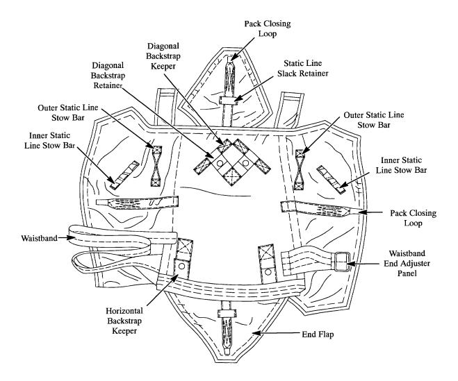
**Deployment Bag.** The T-10C/T-10D parachute is packed in the deployment bag. The deployment bag is constructed of 8.2-ounce cotton sateen cloth. These bags differ in the attachment of a static line, standard (A) and Universal Static Line (USL) (B).
