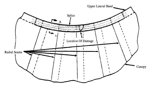
Damage Extending Into Radial Seam
