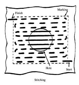
c. Turn the material and weave the needle and thread back and forth across the stitching made in b., above, until the hole is completely darned.
