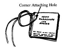
Passing Lacing Loose Ends Through Corner Attaching Hole
