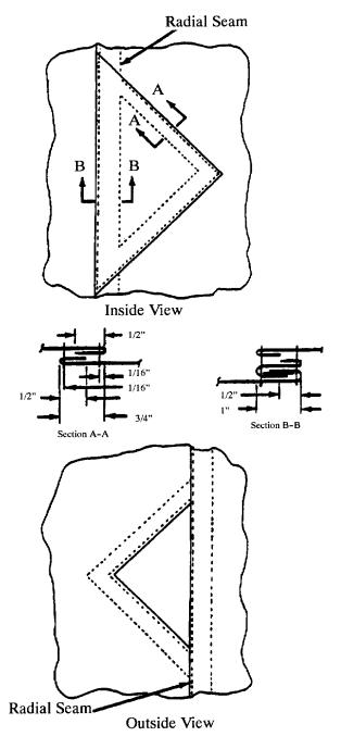
E) Triangular Patch Including Radial Seam
