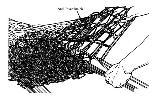
4. Start with line number 16 in the right hand. Pick up line 17 with the left hand and lift straight up until slack is removed from the lower lateral band. With a smooth continuous movement, bring the left hand over the head. When the gore inflates, place line 17 on top of line 16. Make certain the V-tabs are facing down and that the gore material folds to the right side.
