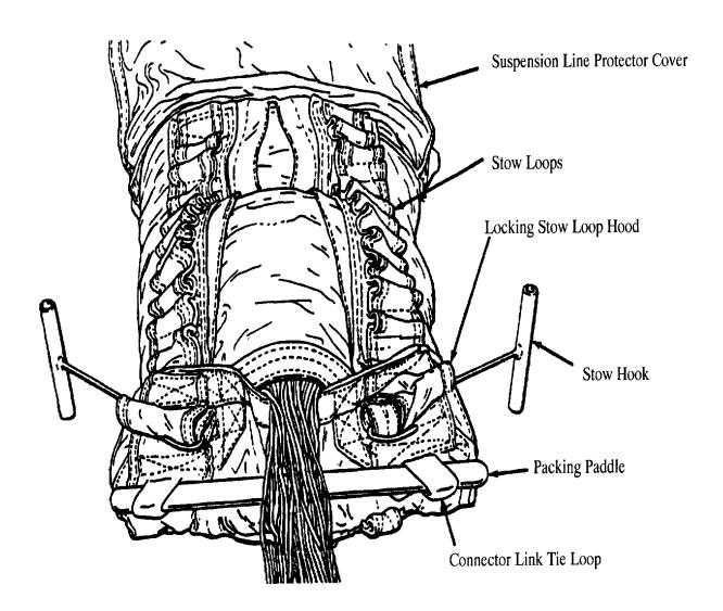
3. Grasp all the suspension lines and form a loop that reaches from the center of the deployment bag to 2-inches beyond the hood of the locking stow loop.
