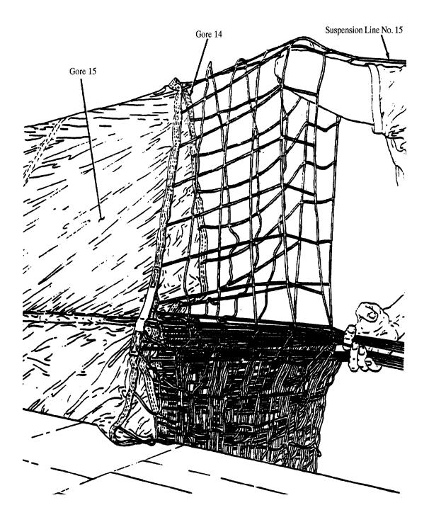
9. Insert the two groups of lines into a line separator, with the left group of lines in the left slot and the right group of lines in the right slot.
