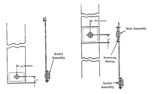
(1) Cut the fabric for the socket and stud assemblies; use a mallet and lead cutter block, and an appropriate sized double- or single-bow cutter.
