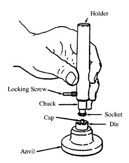
B Hand-Held Tools With Snap Fastener Components Prepared For Use
