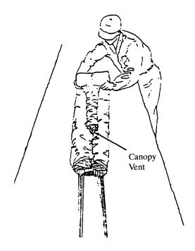
6. Continue rolling the canopy toward the lower end of the suspension lines and risers, if applicable. Locate the lines and riser webbing around the center of the roll.
