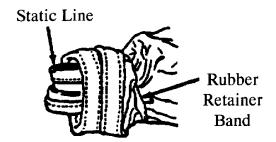
3. For the USL, double a 36-inch length of Type I, ¼-inch cotton webbing. Pass one end of the doubled webbing through both plies of the static line buffer loop, through the bridle loop of the canopy, and back through both plies of the static line buffer loop.
