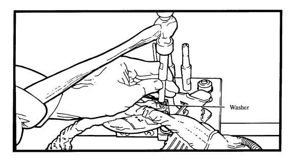
i. Roll the flare, using the proper punch. Remove the assembly from the holding tool and check to assure the lever rotates freely.
