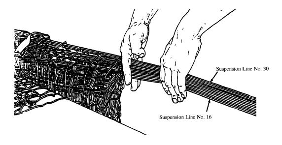
7. Rotate this group of lines clockwise until the fingers are tilted slightly upward, so that line 30 is on the bottom and line 16 is on top.
