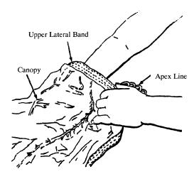
2. Bring the canopy out the skirt, between two adjacent suspension lines.
