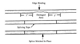
b. Fold-under each end ¼-inch, center the binding over the damaged area, and stitch into place using a medium-duty sewing machine, size E nylon thread, and 7 to 11 stitches per inch. Overstitch the ends of the splice at least ½-inch.
