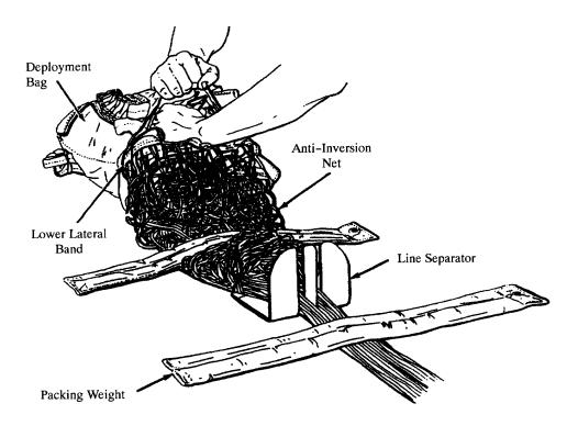
5. With the middle finger of the right hand placed between the left and right group of suspension lines, grasp the anti-inversion net.
