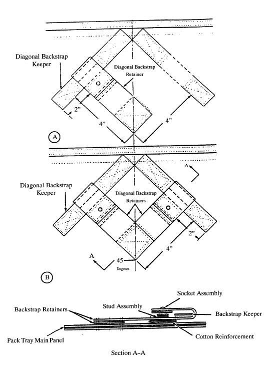
h. Position a new horizontal back-strap retainer as shown below. Sew the retainer in place using a heavy-duty sewing machine, size 3 nylon thread, 5 to 8 stitches per inch, and a box-X-stitch formation.
