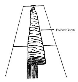
3. CHAIN the suspension lines and S-fold the chained lines on top of the applicable parachute pack.
