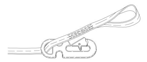
c. Pass the top of the snap hook through the static line loop.
