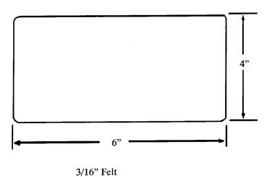
c. Cut two pieces of olive green, type III nylon cloth, 6-inches-long and 4-inches-wide. Round all the corners on a ¼-inch radius.
