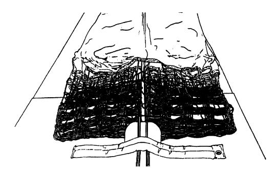
14. Dress the bottom gores by pulling gently on the left and right sides of the canopy; move from the lower lateral band to the apex.
