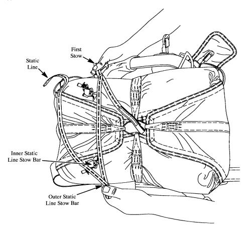
b. Fold remaining static line in half, and rotate it a quarter-turn counterclockwise. Pass the folded end through the static line slack retainer. After hooking the static line snap hook to the static line pack opening loop, pass the folded end under the stowed line. Pull the static line taut, and slip the folded end of the line under the lower end flap.
