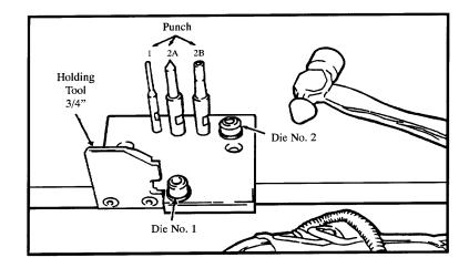
a. Install the female fitting on the holding tool and secure by closing the locking arm. Assure the head of the assembly pin is seated in the No. 1 die fitting.
