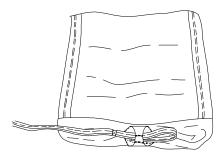
b. Pass the 3½-inch loop end of the 15-foot static line through the 6-inch buffer loop, counterclockwise, until a taut girth-hitch is formed.
