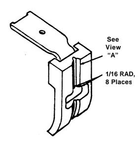
Modified Presser Foot For Anti-Inversion Net Repairs
