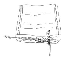
c. Secure the static line to the deployment bag.
