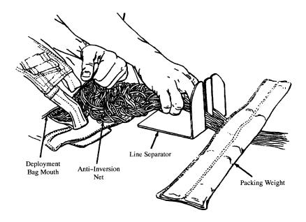
6. With the left hand, move the packing weight and line separator. Then place the left hand on the mouth of the deployment bag; with the right hand, slide the anti-inversion net into the center of the deployment bag.
