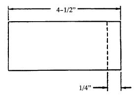
d. Fold both ends over along the row of stitching; stitch through the ends and one layer of the loop  $\frac{1}{16}$  inch from the webbing ends. Use a light-duty sewing machine, size E nylon thread, and 7 to 11 stitches per inch.
