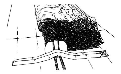
13. Apply additional tension to the suspension lines, and flip the left group of gores (top half) to the left side of the table.
