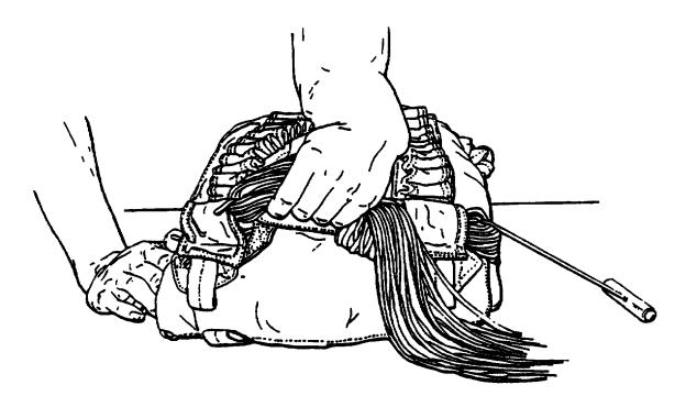
8. Pull the suspension line loop through the left locking stow loop. The enclosures of the stow should extend 2-inches beyond the hoods of the locking stow loop.
