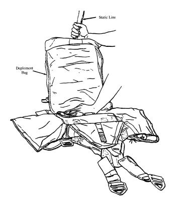
4. Remove twists from the static line and fold the static line across the deployment bag so that the packopening loop is up and in the center of the bag. Fold remaining sleeve portion under the upper end of the deployment bag.
