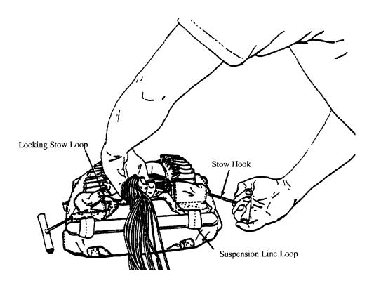
5. Pull the suspension line loop through the right locking stow loop. The ends of the stow should extend 2-inches beyond the hood of the locking stow loop.
