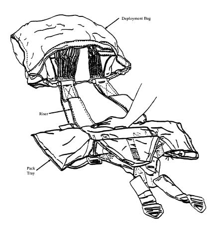
2. Slip risers through riser slots in upper flap of the pack tray. U-fold the risers onto the pack tray.
