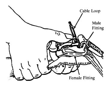
e. Position the cable loop around the latch.
