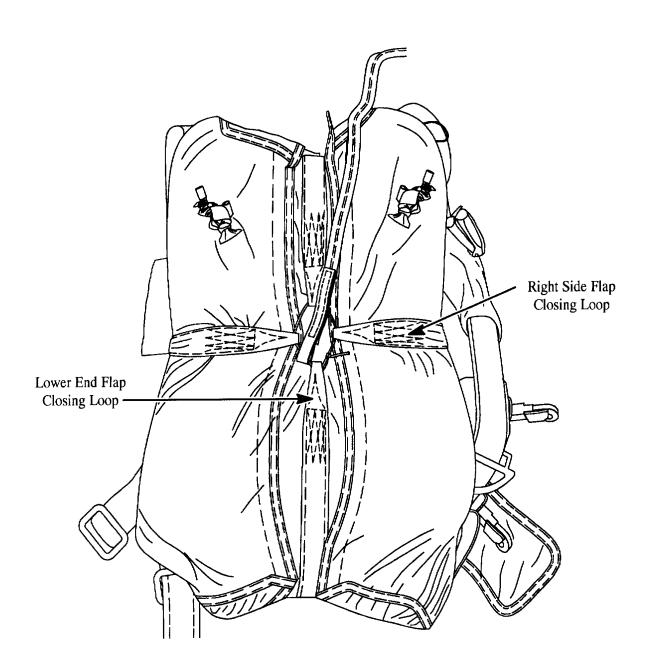
7. Using a packing paddle, insert flaps and dress the pack. The pack tray is now closed.
