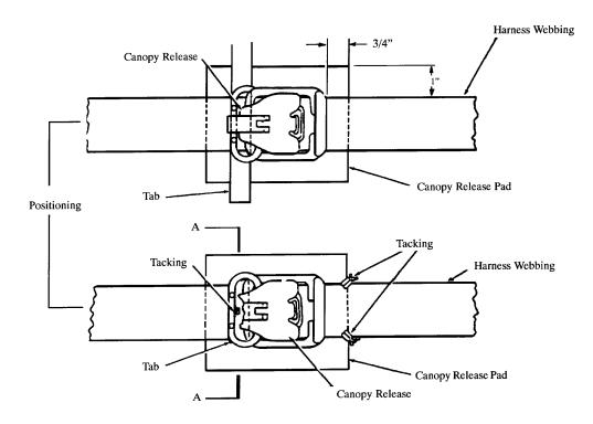
j. Fold the tab around the harness webbing; hand tack the ends of the tab together with two-turns of doubled and waxed tape, lacing and tying.
