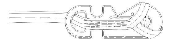
d. Continue passing the snap hook through the static line loop; pull the excess static line back through the opening in the base of the snap hook until the loop is past the snap hook opening.
