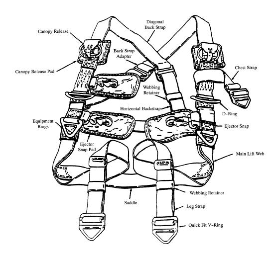
**Riser Assembly.** Each of the two riser assemblies is 30-inches long (finished length) and constructed of type XIII nylon webbing, with the male canopy release fitting permanently attached. The two ends of each riser are attached to the suspension line connector links.
