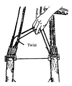
(1) To remove twists, grasp top and bottom inside lines (lines 1 and 30, and 15 and 16) at skirt of canopy and trace them to connector links.
