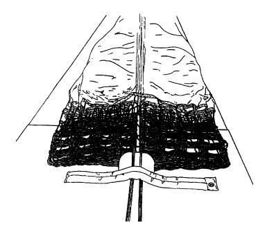
18. Raise the top radial tape, No.30, and check for a clear channel.
