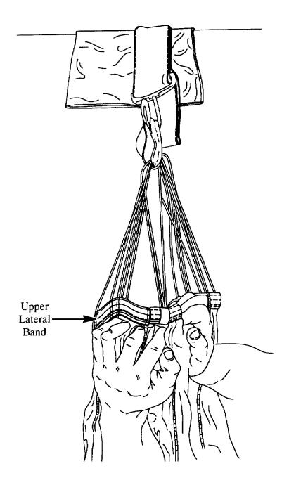
2. Move to the lower end of the table and apply first tension on the parachute until the suspension lines are taut and rise off the table.
