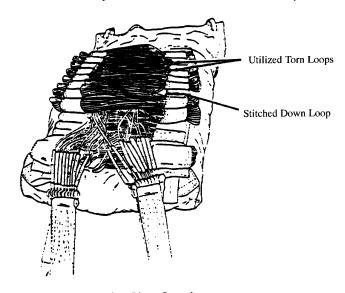
Suspension Lines Stowed Utilizing Torn Stow Loops
