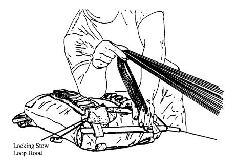
4. Insert the right stow hook through the loop formed by the suspension lines. Ensure the stow hook is around all of the suspension lines.
