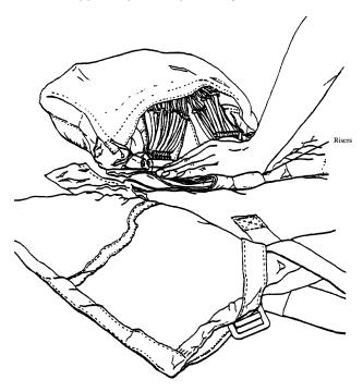
3. While holding folded risers in place, grasp the static line at the end of the deployment bag, and rotate the bag onto the pack tray.
