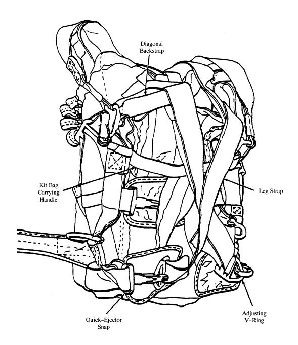
3. Grasp the saddle and pull straight up. Take the waistband through the saddle and completely around the harness located under the kit bag (pull tightly). Thread the waistband back through the saddle, into the waistband adjuster, then back through the waistband adjuster, forming a quick-release.
