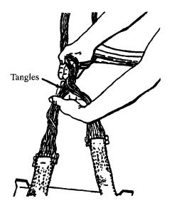
(2) Reach through the opening, created by lifting the suspension lines, with the right hand.
