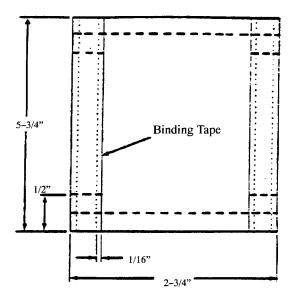
d. Position the prepared locking stow loop hooked in the same place as the one removed. Stitch the hood in place using a light-duty sewing machine, size E, nylon thread, and 7 to 11 stitches per inch in two box-X formations. The finished hood should not exceed 3-inches in width.
