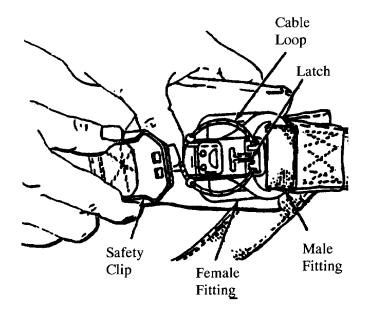
f. Fit the heel of the safety clip into the slot of the latch.
