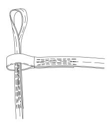
c. Pass the snap hook of the 5-foot extension through the 3½-inch loop, on the 15-foot static line.
