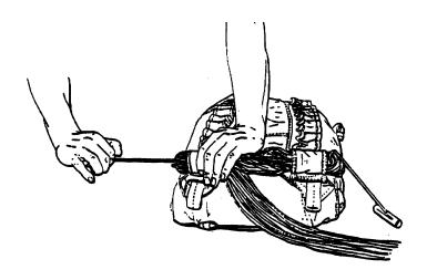
9. Extend the suspension lines to the upper right corner of the deployment bag. Form the first regular stow.
