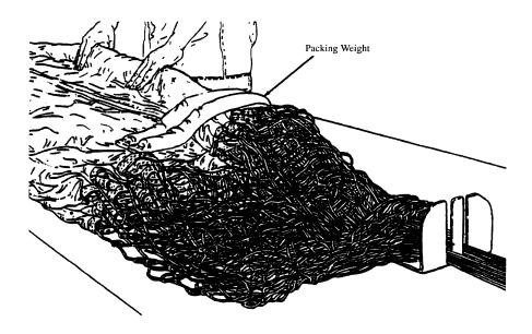
5. Place the second packing weight. Continue folding until you reach approximately 48-inches from the apex. Then place the third packing weight.
