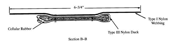
i. Position the pad under the canopy release as shown.
