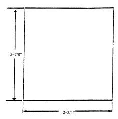
c. Bind the  $5^7/_8$ -inch edges with  $\frac{3}{4}$ -inch, type III, cotton tape; turn-under ends of the tape  $\frac{1}{2}$ -inch. Using a light-duty sewing machine, size E, nylon thread, and 7 to 11 stitches per inch, stitch the binding tape with two rows of stitches.
