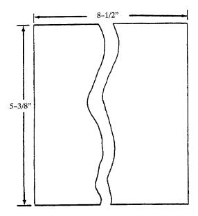
c. Fold the cloth in half; align the  $5^3/_8$ -inch side, and stitch ½-inch from the edge on the  $5^3/_8$ -inch side, and one of the  $4\frac{1}{4}$ -inch sides. Use a light-duty sewing machine, size E nylon thread, and 7 to 11 stitches per inch.
