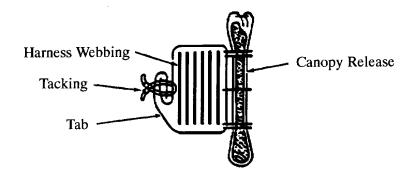
m. Tie the ends of the lacing with a surgeon's knot and a locking knot.
