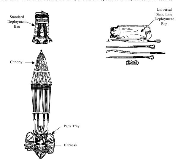
**Equipment Name.** T-10C Troop Back Parachute Assembly, 35-Foot Diameter, and T-10D Troop Back Parachute Assembly, 35-Foot Diameter.
