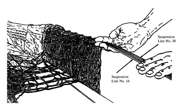
8. Starting with line 1, fold the left group of gores using the same movement as in step 3., above. Continue folding the gores until you reach suspension line No.14. Raise suspension line No.15 and drape the last gore on the left and the next to last gore on the right.
