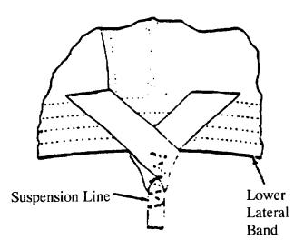
d. Position the webbing on the damaged area. Using a light-duty sewing machine, and size E, nylon thread, sew the webbing in place with four continuous rows of stitching, 7 to 11 stitches per inch. Overstitch the ends of the webbing by 2-inches.
