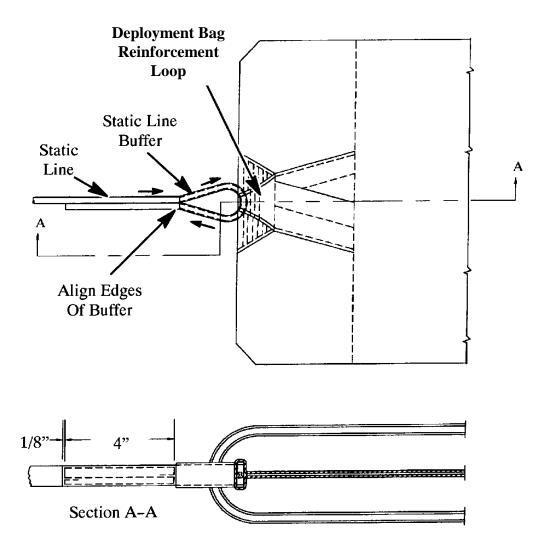
(3) Align the two ends of the buffer and stitch the static line in place; use a heavy-duty sewing machine, size 6, nylon cord, 5 to 8 stitches per inch, and a static line stitch formation 4-inches long.
