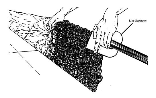
11. Turn the line separator counterclockwise so the base is down, and slide it back on the table.
