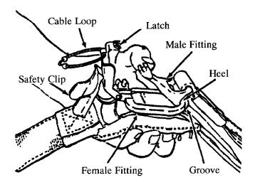
c. Fit toe of male fitting into slot of female fitting, close latch. Ensure that the latch is securely locked.
